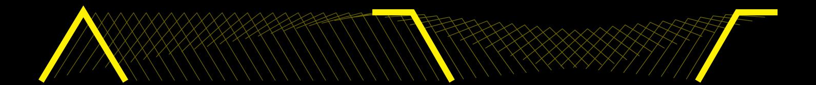
The Colour act as a three input crossfader. It transitions smoothly from band pass to low pass to high pass.
