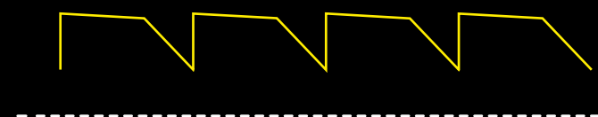
10Vpp saw wave, ~9V offset, DC mode
